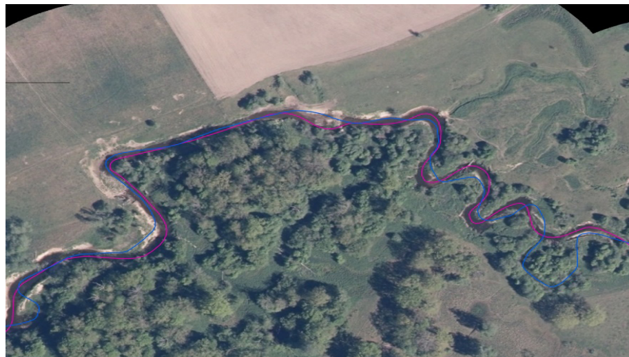
Figure 4. Changes in the axial line of the river bed: GDR10LT data (blue) – in 2003; data compiled by drone (red) – in 2022
