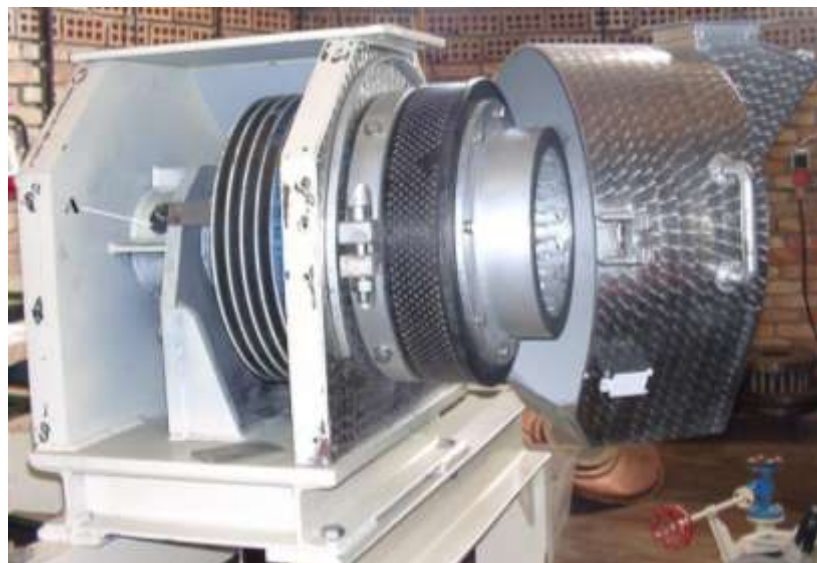
Fig. 5. View of the ring working system of the PD-1 pellet mill; A-place where a set of tensometers for the measurement of matrix torque is stuck on
